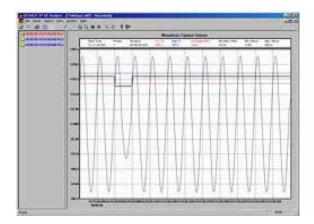
Voltage drop - The trigger is on voltage RMS value, the resolution is 1 cycle. 2+10 waves before and after the trigger are represented, the sampling is 32 samples / cycle.
