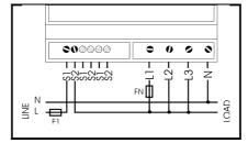
WIRING DIAGRAM: 3 PHASES - 3 WIRES / 3 CURRENT TRANSFORMERS (3.3.3) (on request)
